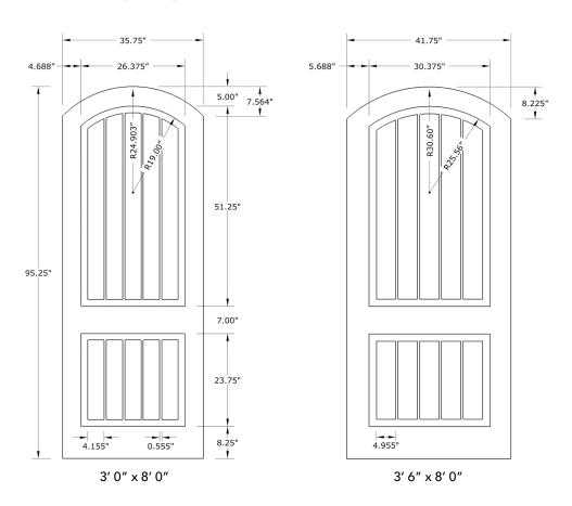
NOTE: BY REQUEST, DOOR HEIGHT COMES IN VARYING DIMENSIONS TO A MINIMUM OF 95". EXCESS WILL BE TAKEN FROM BOTTOM RAIL. ALL OTHER DIMENSIONS WILL REMAIN THE SAME.
